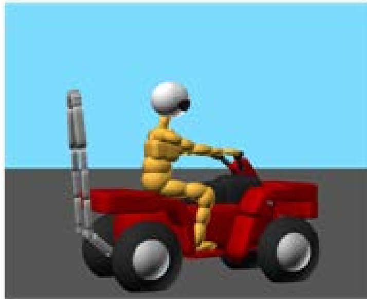
26 27 28 Figure 1. Image of the test-calibrated computer simulation model of the MATD on the 29 TRX 350 ATV with CPD and full face helmet 30
